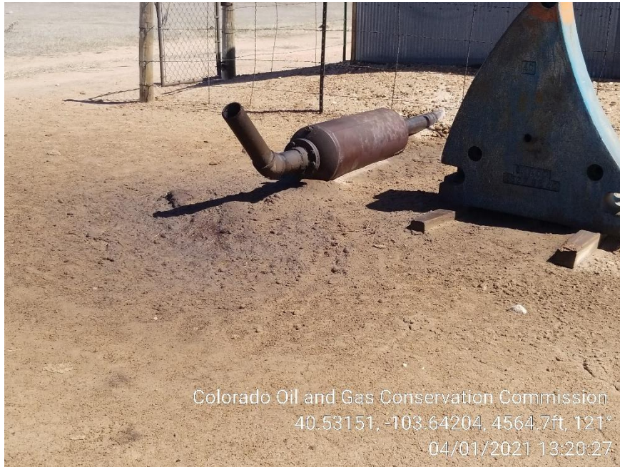
Photo 5 – Stained Soil at Gas Engine Exhaust
