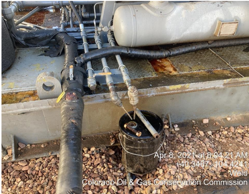
Photo #7 Mechanical conditions/ Oily Waste
