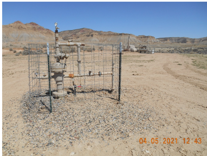
Wellhead with fence.
