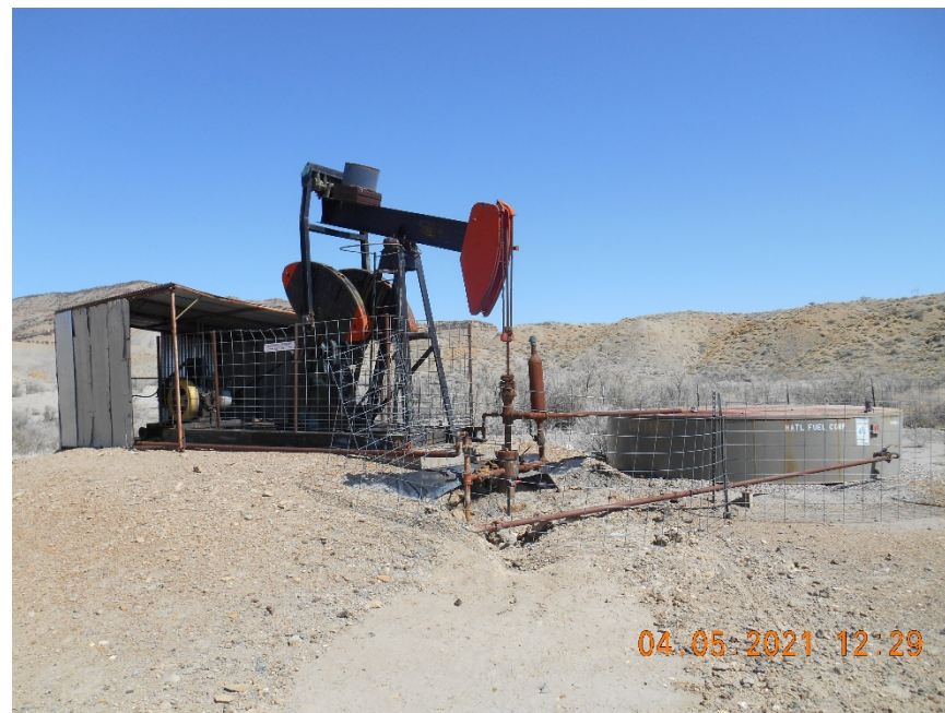
Wellhead with Pump Jack.
