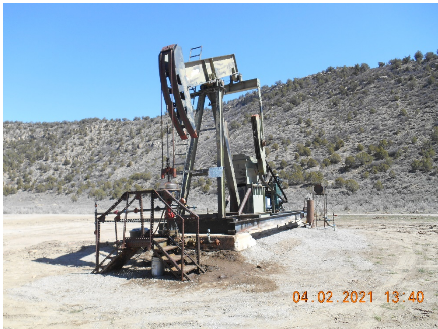
Wellhead with pumpjack
