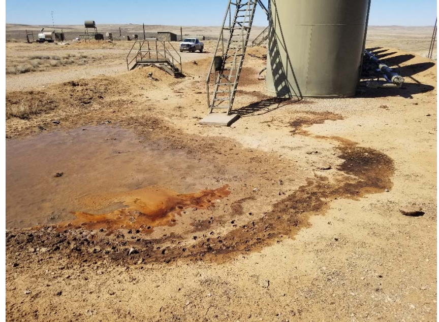
Photo 18. Stained soil in berm. Animal footprints (pronghorn and deer) visible around perimeter of fluid puddle.
