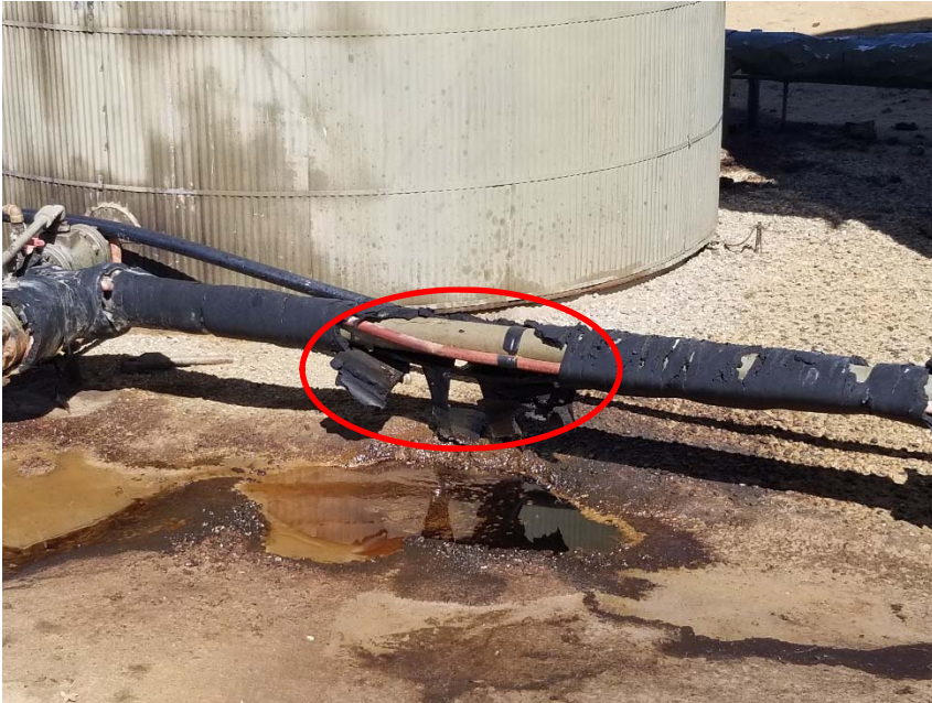
Photo 7. Active leak, ongoing release from flowline.
