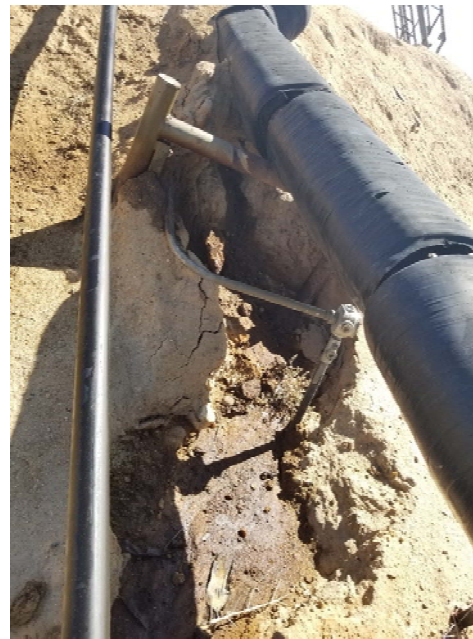
Photo 10. Berm breach. Spill leaving location.
