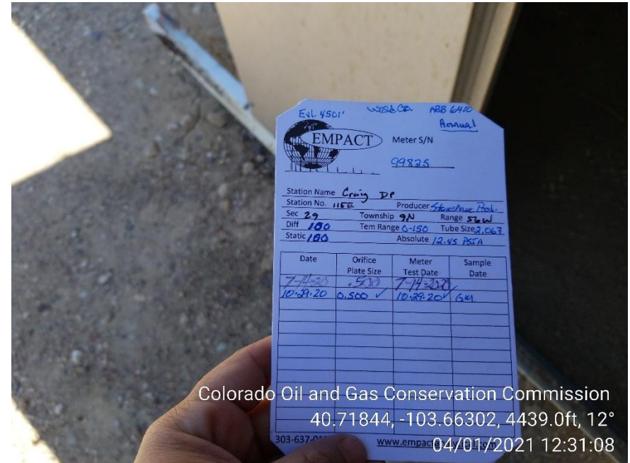
Photo 6 – Gas Meter Calibration Card is up to date
