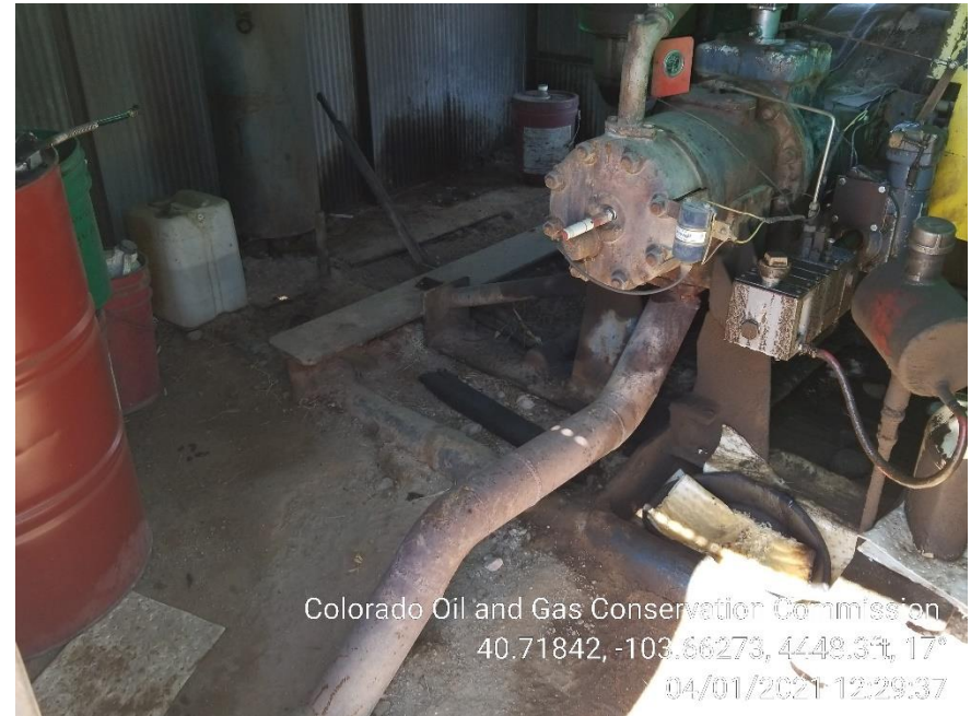
Photo 8 – Stained Soil at Gas Engine
