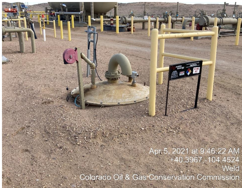
Photo #5 Inadequate Berms
