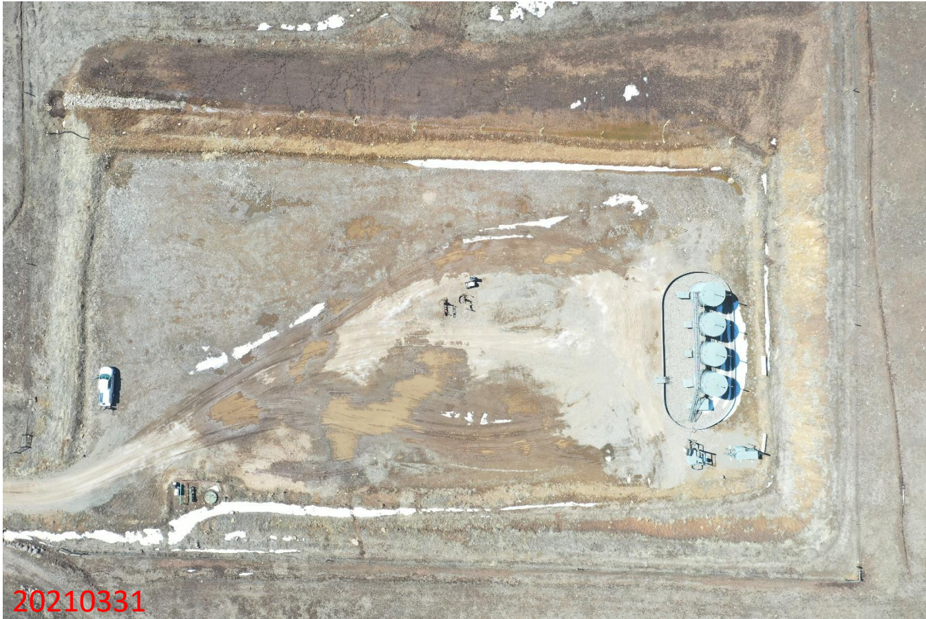
Photo 1: Photo taken with a small unmanned aerial system. Photo shows aerial image/overview of the Location. Previous inspection required Operator to conduct interim reclamation on areas not needed for production. Photo shows reclamation of areas not needed for production on the Location has not been conducted pursuant to 1003 requirements.
