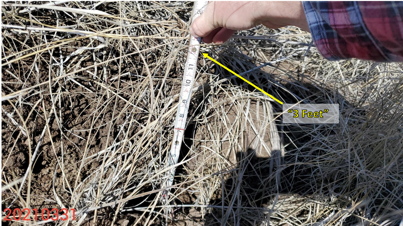
Photo 4: Photo taken from crack on the perimeter of the Location. Photo shows example of areas where cracks on the Location were observed to exceed 30 inches in depth.
