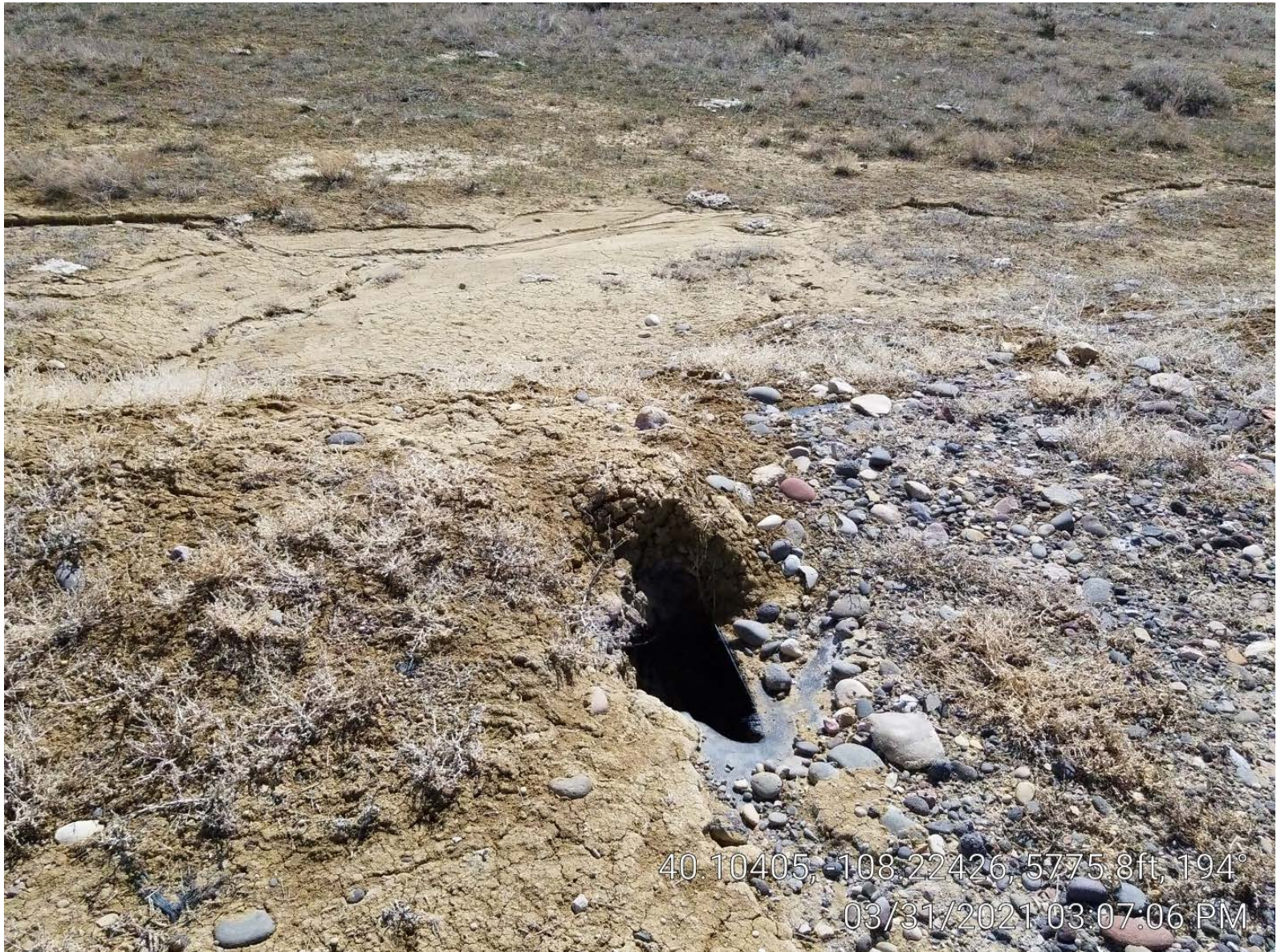
Photo 9. Erosion hole & channel at edge of location.
