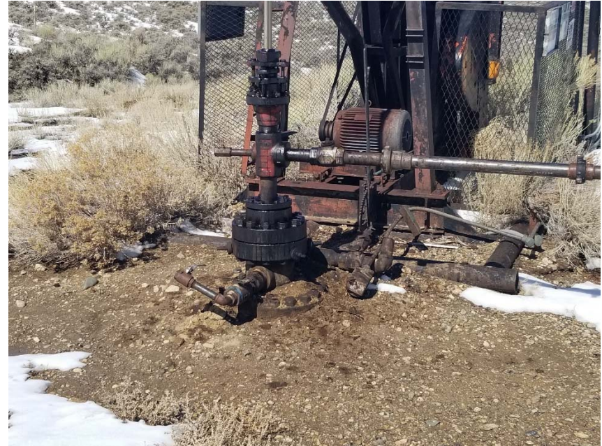
Photo 2. Stained soil at wellhead. No bradenhead access apparent.
