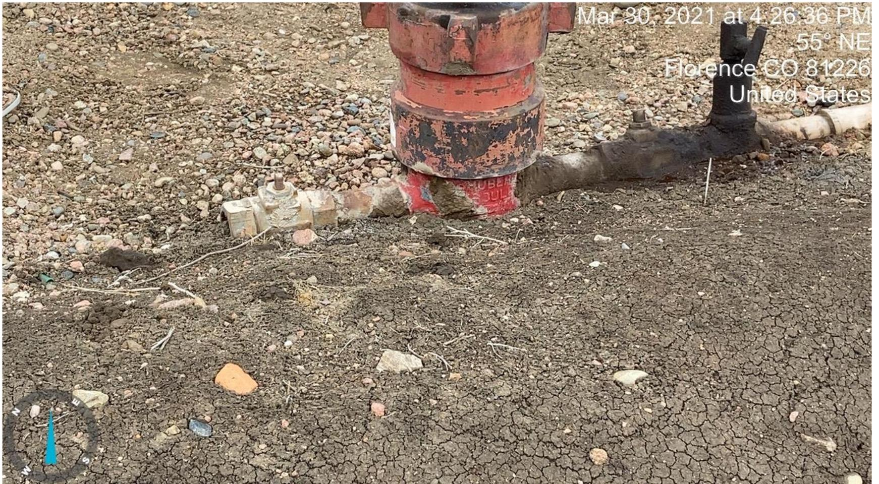
PHOTO 4: BRADENHEAD IS NOT PLUMBED TO SURFACE. **CONTACT AREA ENGINEER FOR GUIDANCE. CA DATE 4-10-21.**
