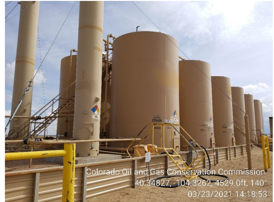
Photo 12 – Tank Battery
