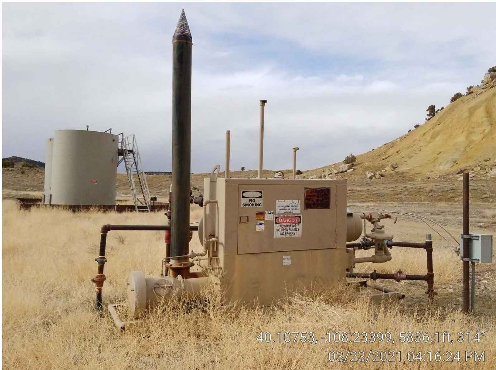
Photo 3. Separator & tanks.
