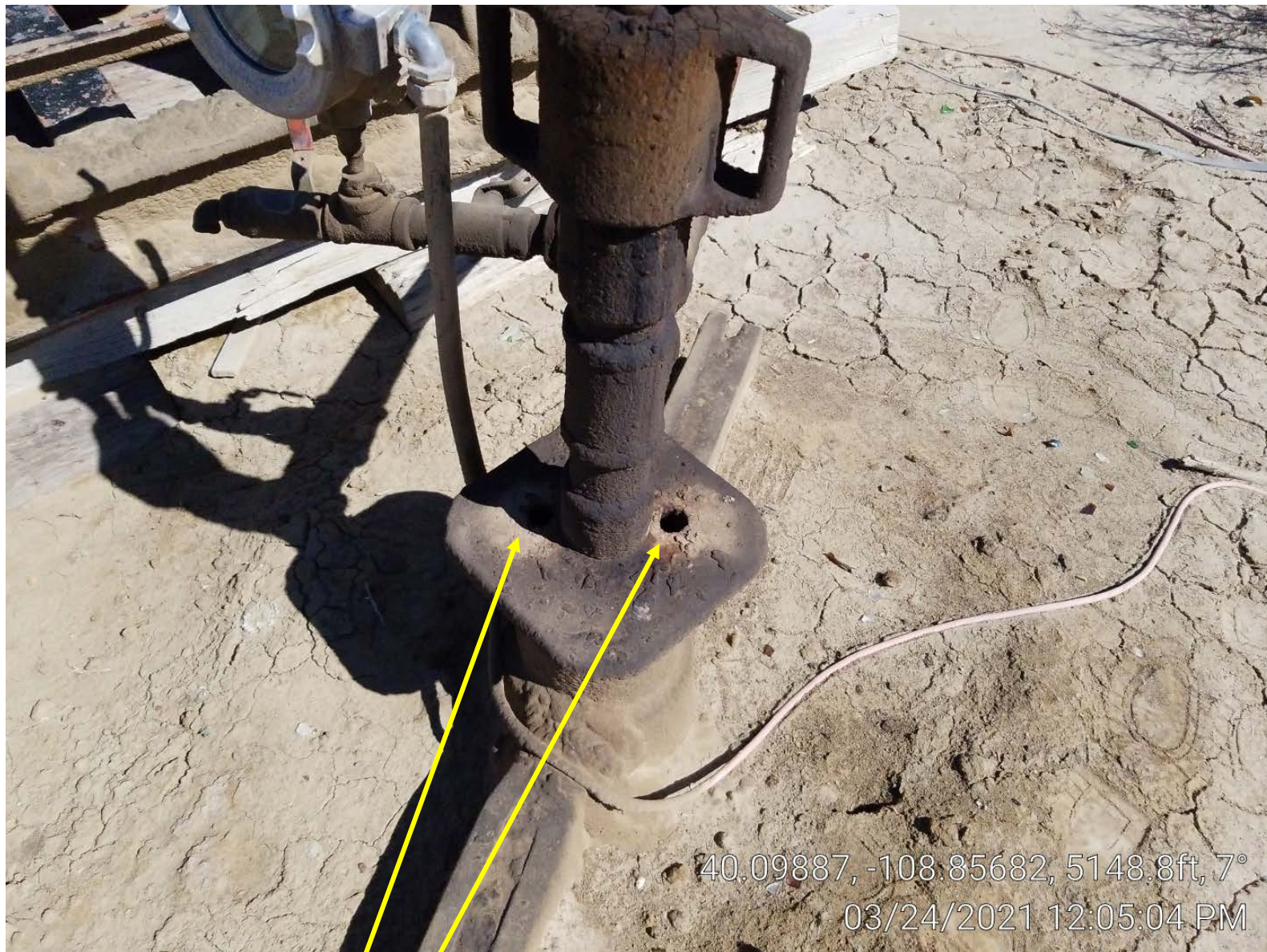
Photo 2. Well with casing venting.
