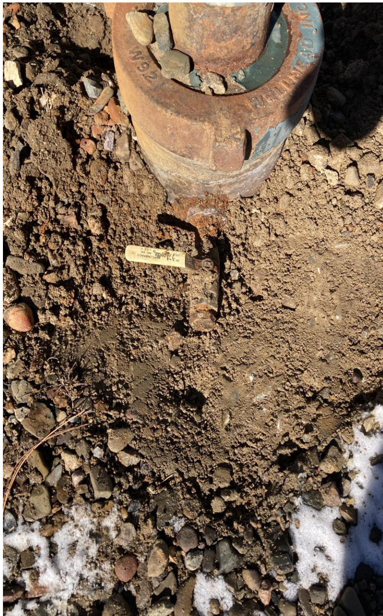
Plumbed bradenhead to surface
