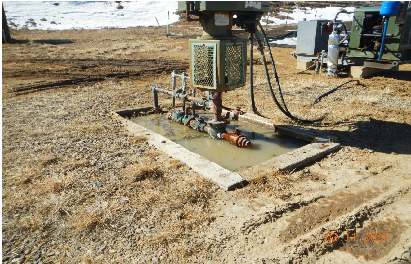
Photo 2. The wellhead is still dripping produced water and needs to be repaired.
