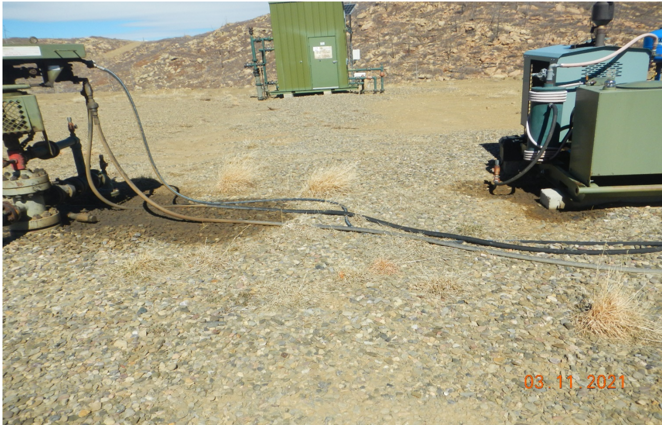
Photo 3. There is oil stained soil at wellhead and engine.
