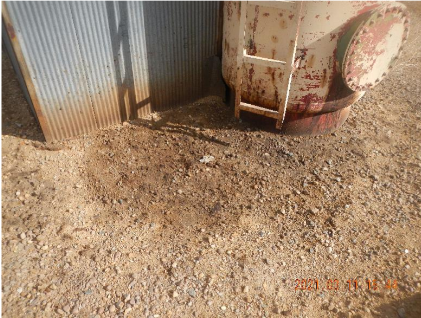
Photo 15: Impacted soil around base of heater treater.
