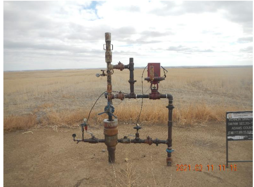
Photo 2: View of wellhead, wellhead tree, and plunger lift system.
