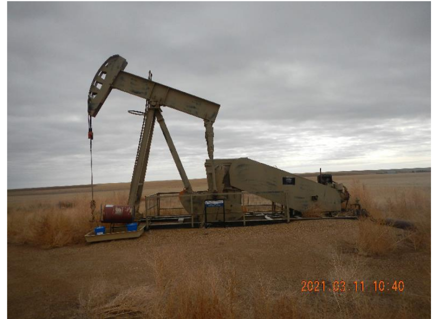
Photo 2: View of pumping unit.
