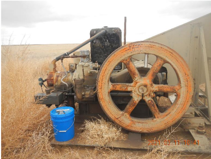
Photo 3: Gas fired prime mover. One of four 5 gallon buckets of mineral spirits at well site.
