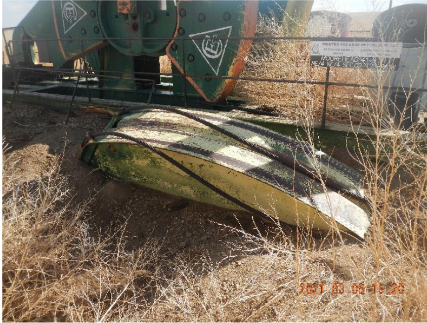
Photo 11: Removed horsehead and bridle beside pumping unit.
