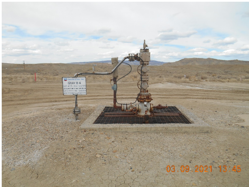
Injection wellhead
