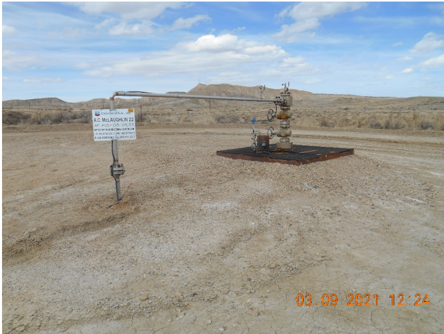
Injection wellhead
