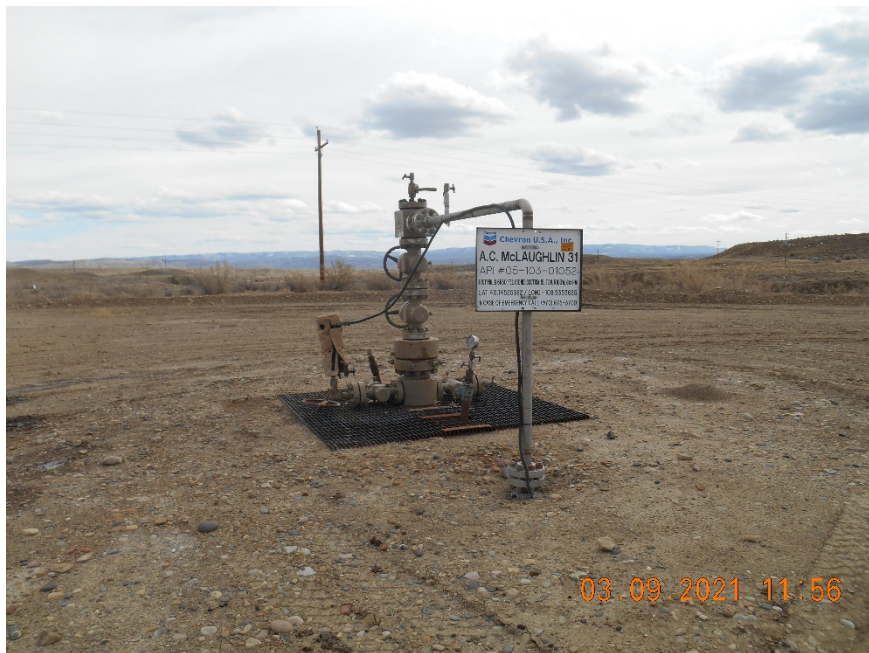
Injection wellhead.
