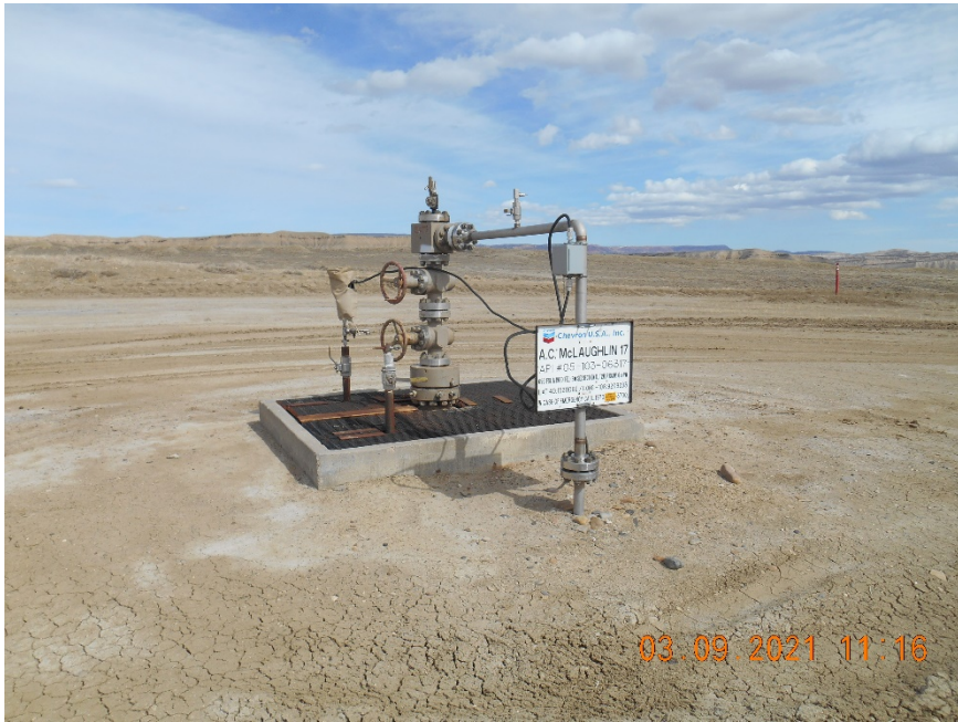
Injection wellhead
