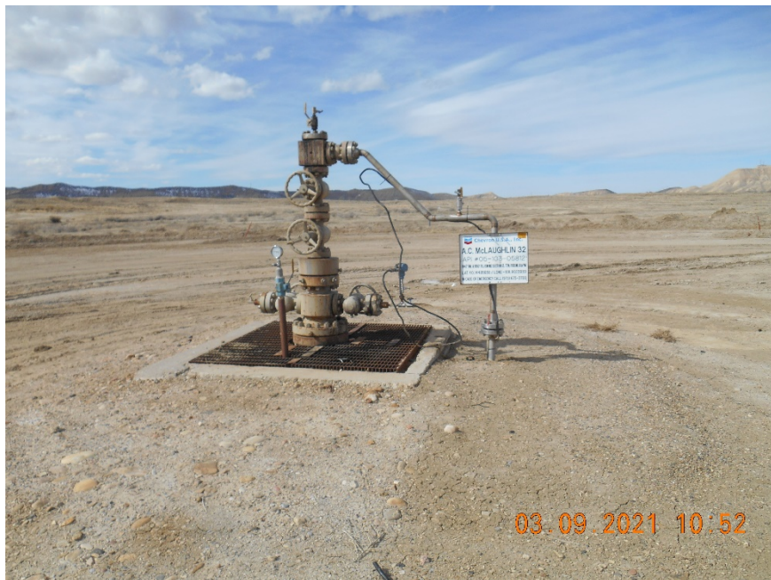
Injection wellhead
