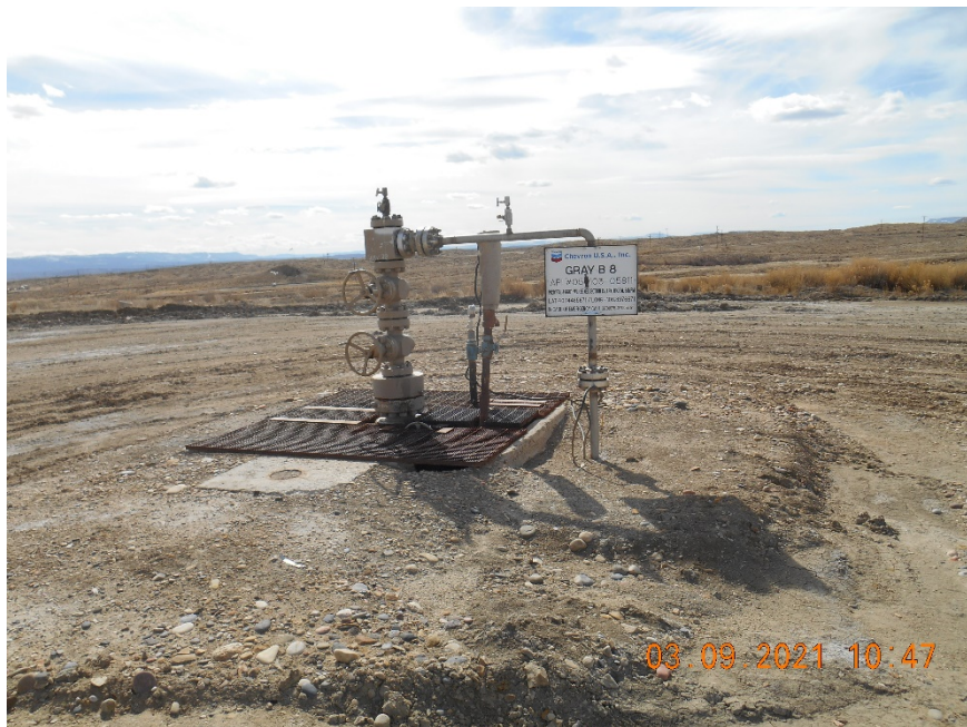
Injection wellhead
