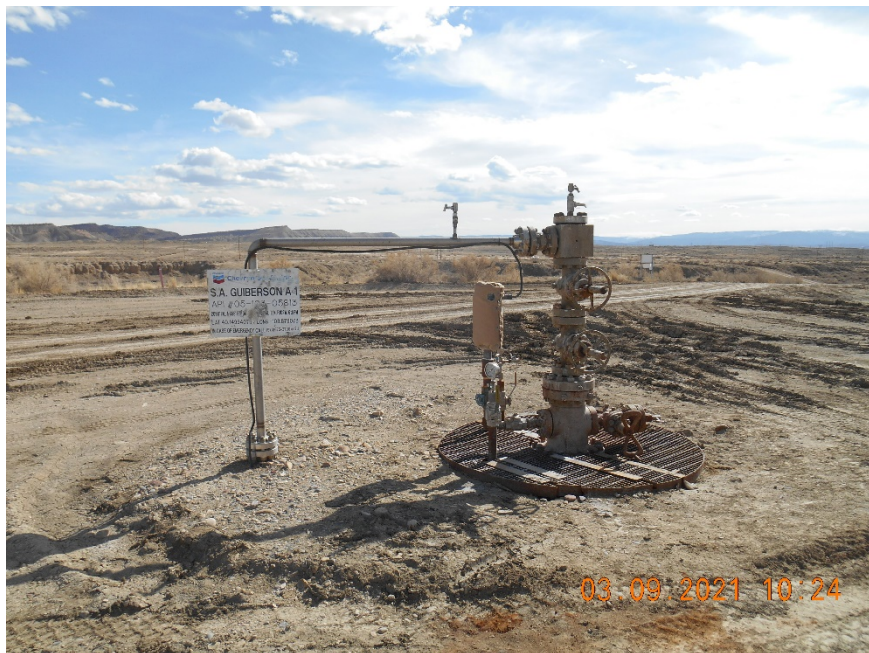
Injection wellhead
