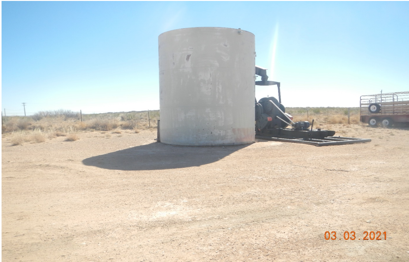
Photo 6. There is a tank and pumpjack at the south side of the location which needs to be removed.
