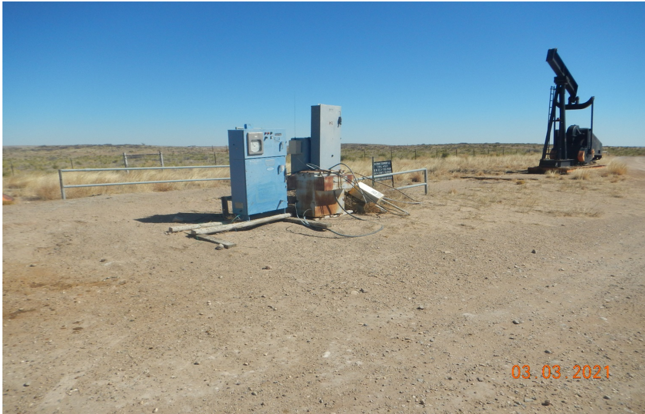
Photo 3. Facing toward the well. The pumpjack has been moved. It appears the well was plugged and abandoned on 11/19/2020.
