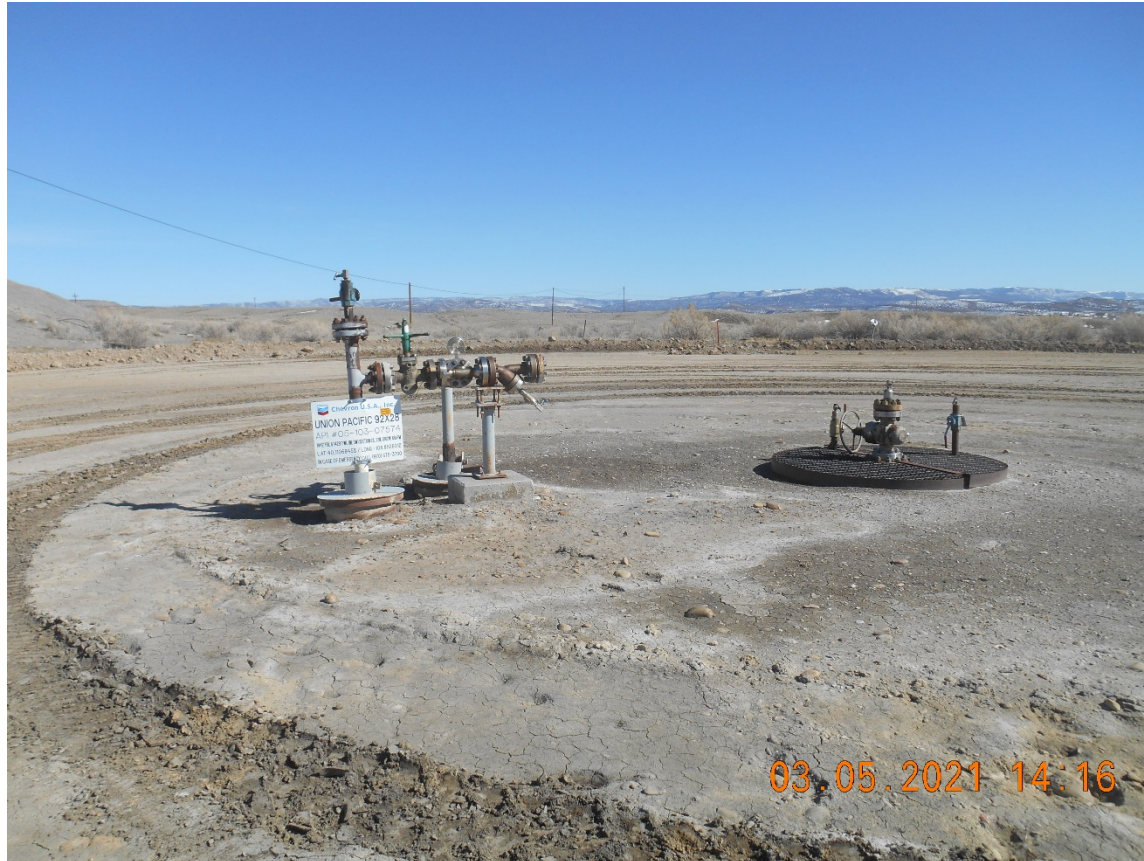
Injection wellhead. Temporarily Abandoned.
