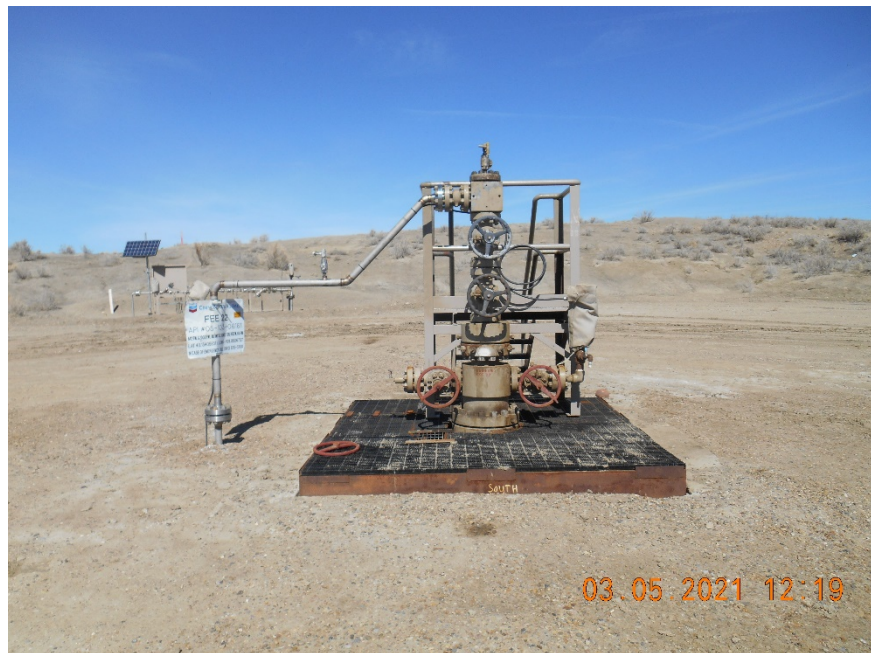
Injection wellhead
