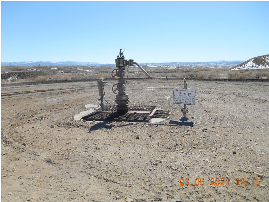
Injection wellhead
