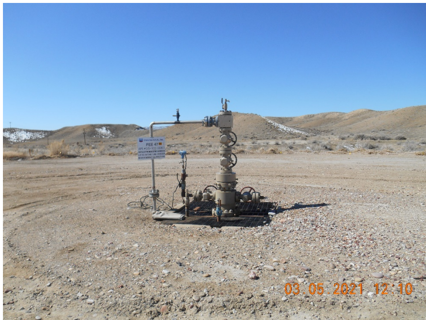
Injection wellhead
