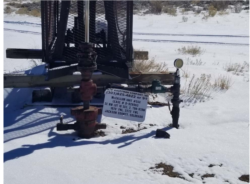
Photo 2. No bradenhead access apparent.
