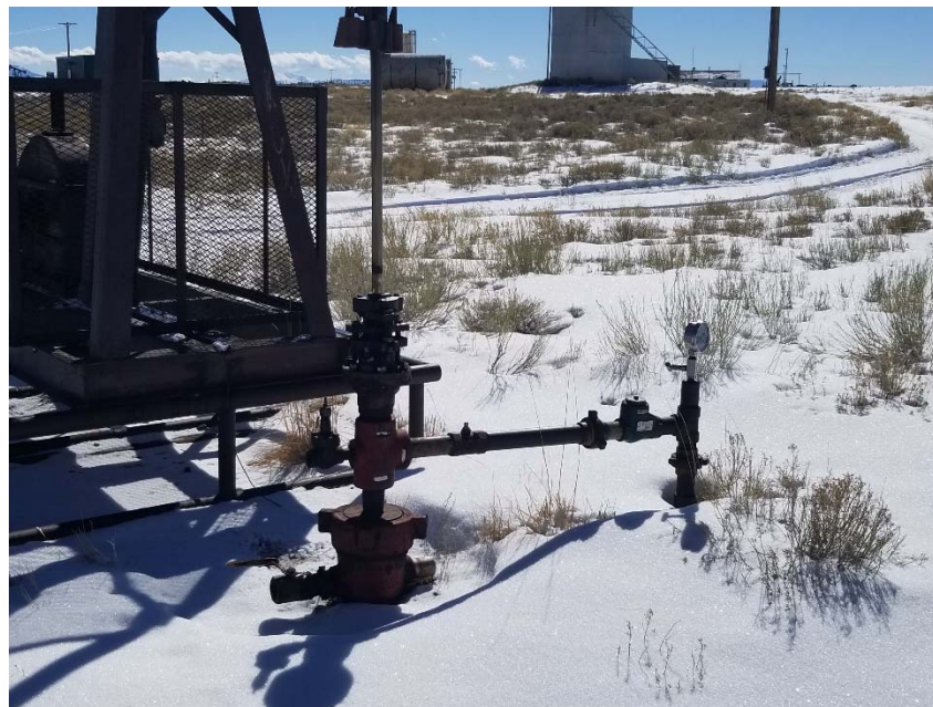
Photo 2. No bradenhead access apparent.
