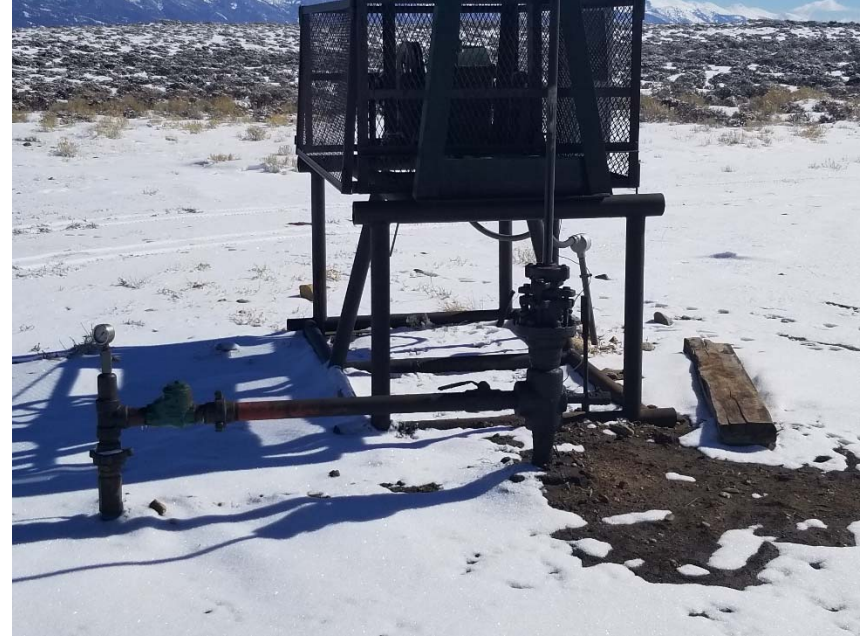
Photo 2. No bradenhead access apparent.
