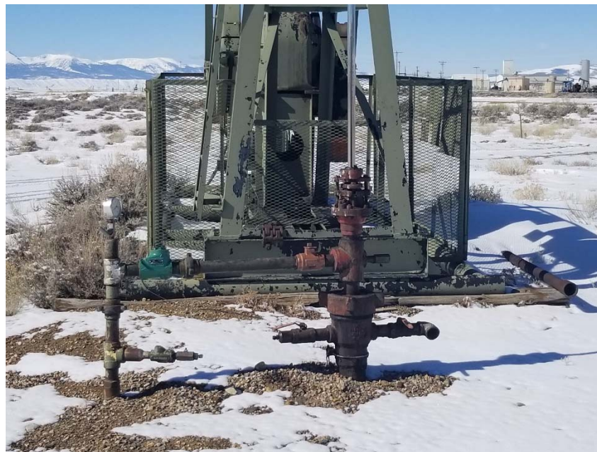
Photo 2. No bradenhead access apparent.
