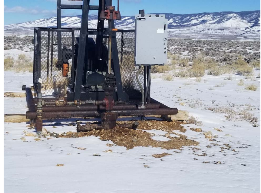
Photo 2. No bradenhead access apparent.
