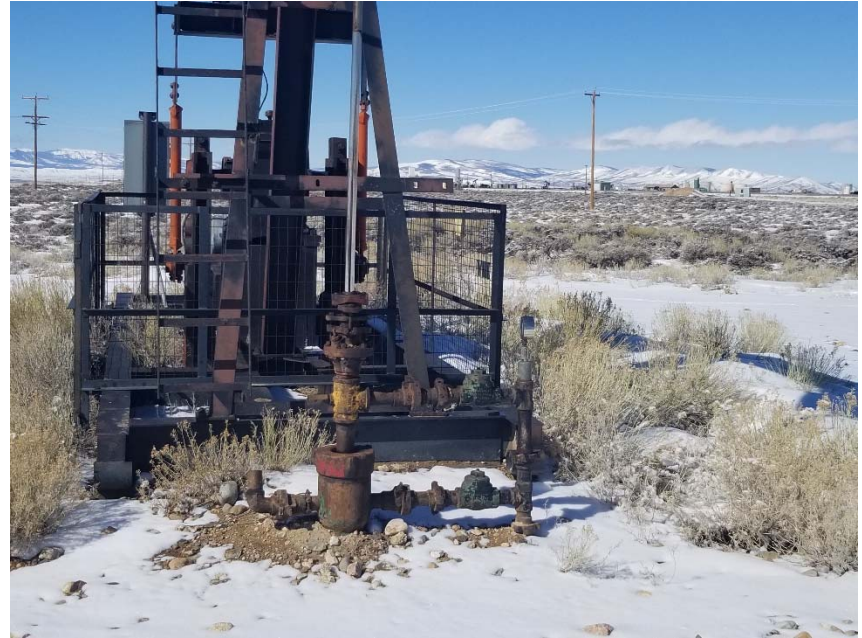
Photo 2. No bradenhead access apparent.
