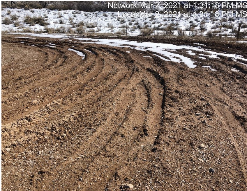
Photo #3036 Rutting present on location due to lack of stabilization
