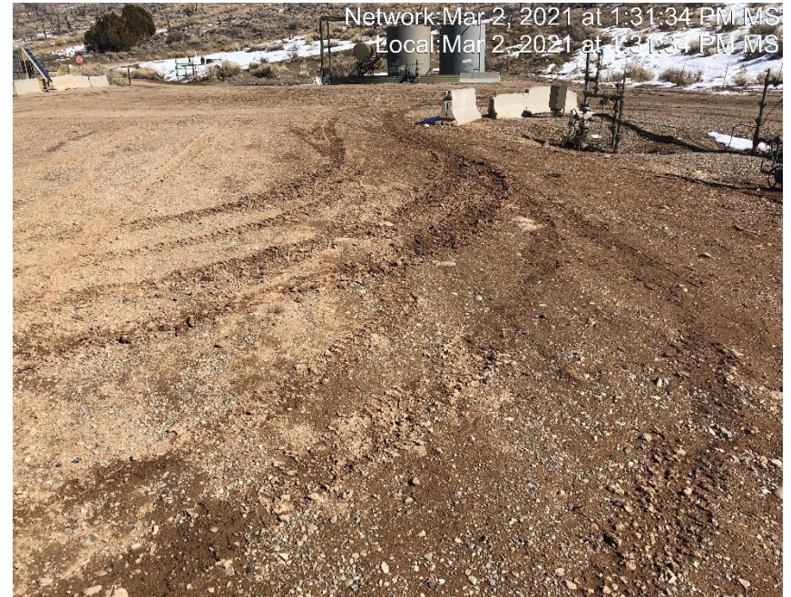
Photo #3037 Rutting present on location due to lack of stabilization
