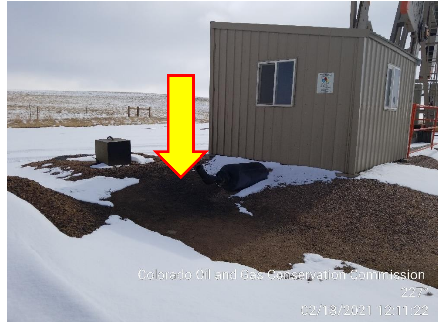
Photo 4 – Stained Soil at Exhaust
