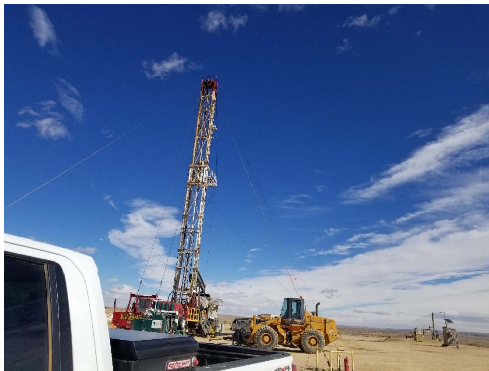
Photo 1. Workover on location.
