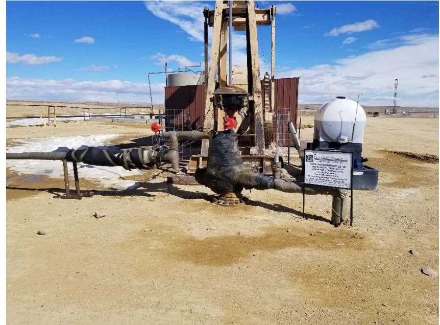
Photo 2. No bradenhead access apparent.
