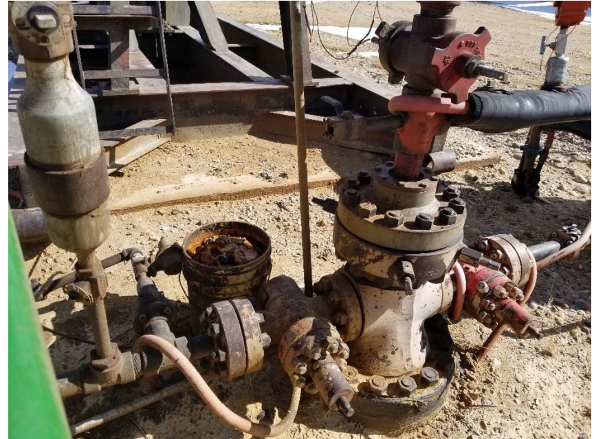
Photo 4. Bucket with oily rags at wellhead.
