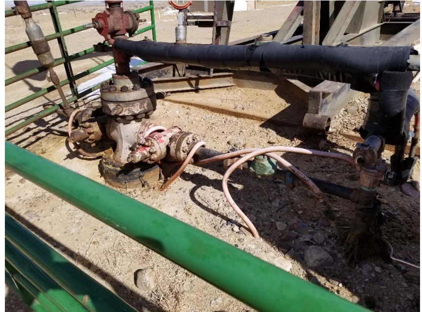
Photo 2. No bradenhead access apparent.
