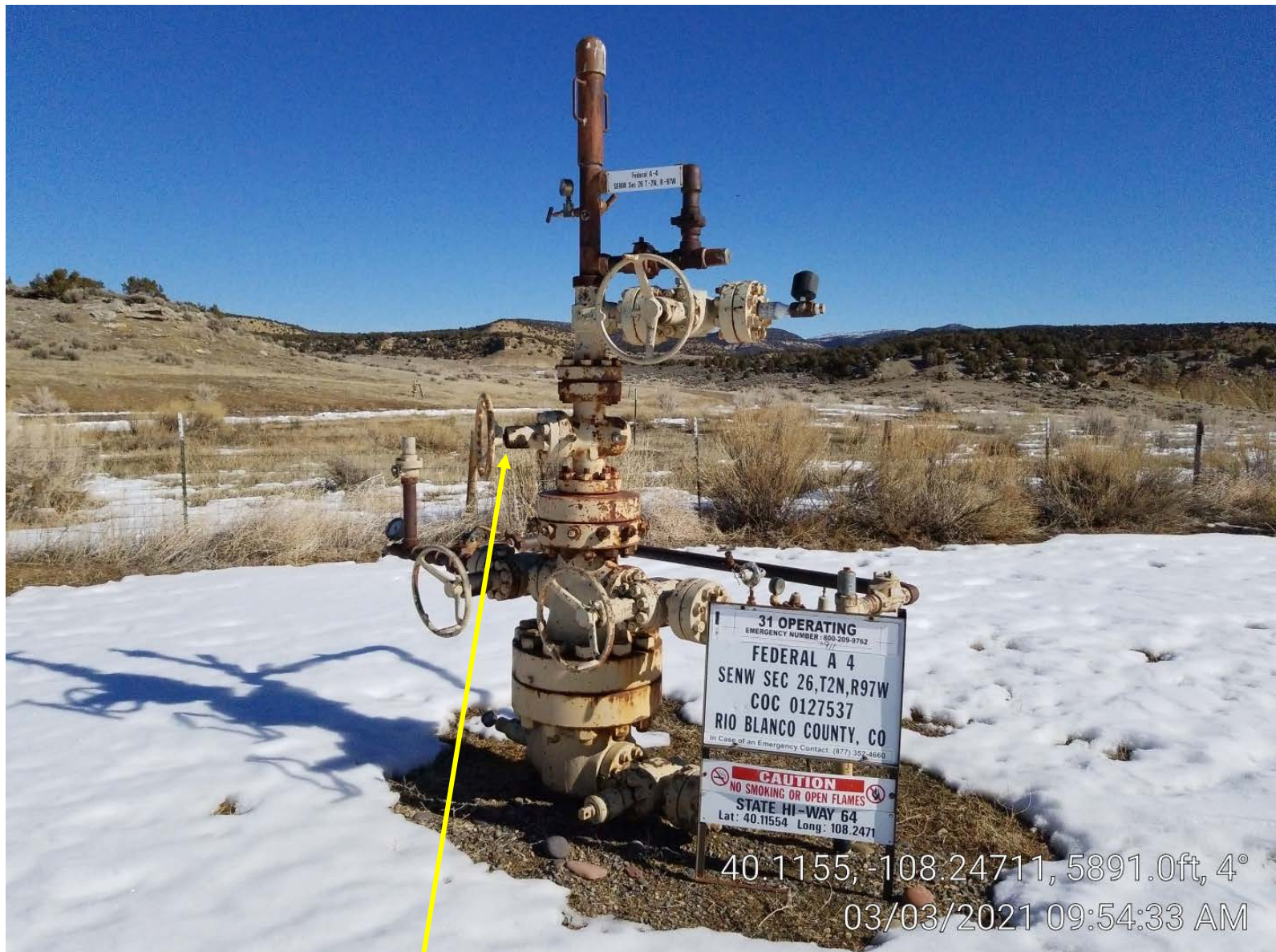
Photo 2. Well with gas leak.
