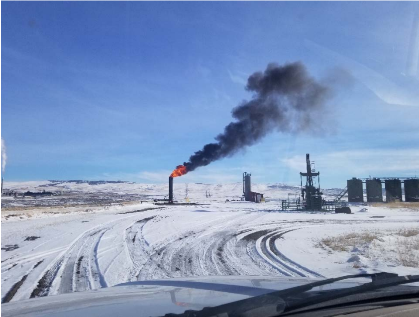
Photo 1. Photo of combustor with flames. Photo taken from entrance to location.
