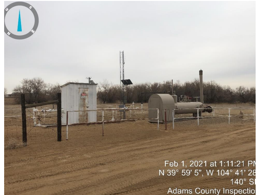
Photo #2 Meter & Separator.
