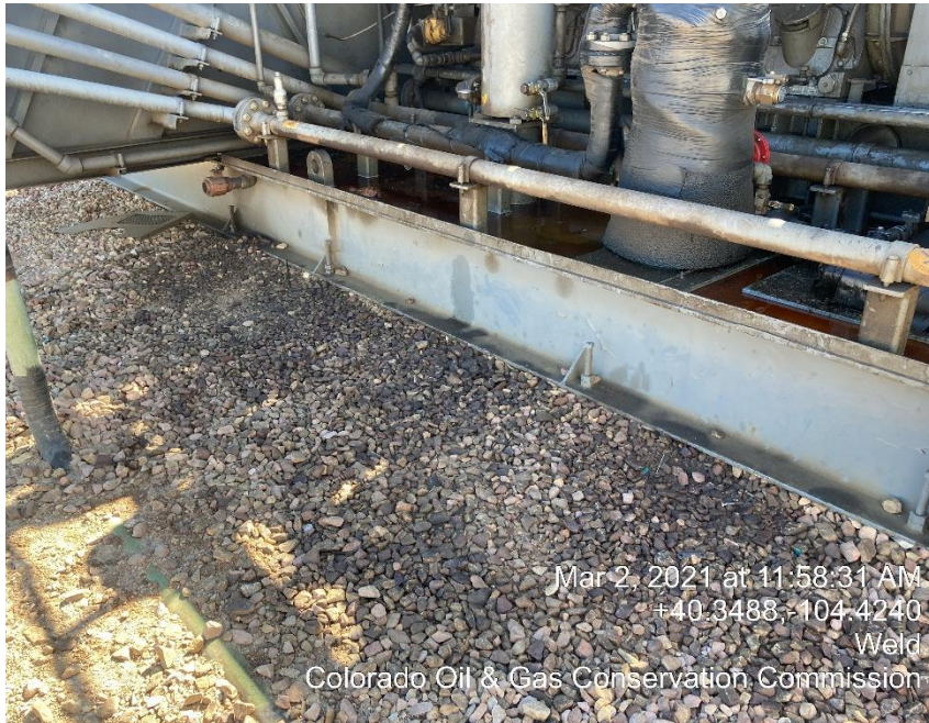
Photo #35 Stained soil/ Oily skid
