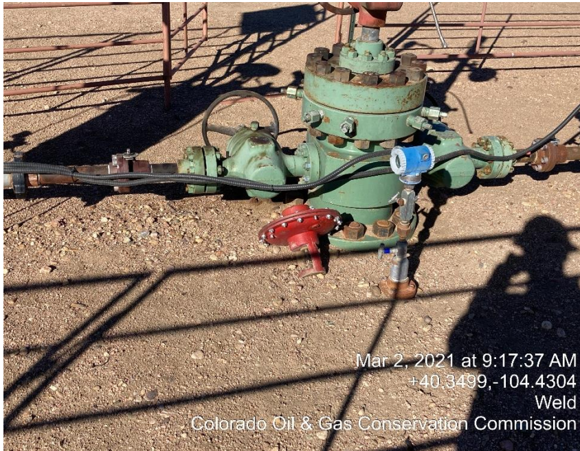
Photo #5 Unused Equipment “motor valve”
