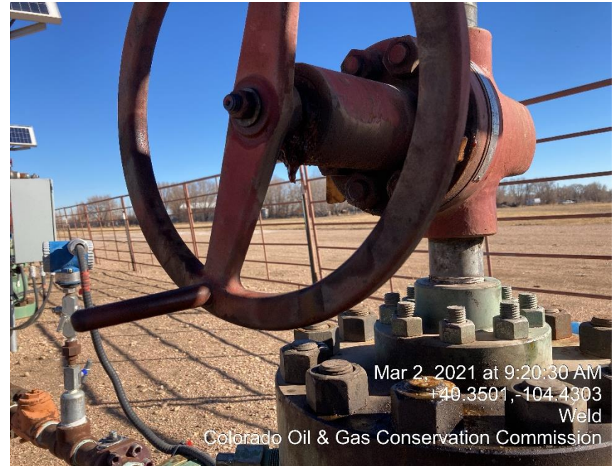
Photo #16 Leaking Master Valve
